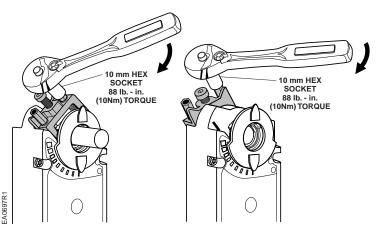
**NOTE:** Keep the shaft in the center of the shaft adapter opening. Apply 7.5 lb-ft (10 Nm) torque maximum.
